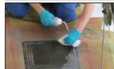
Water break test
