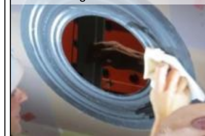
Skin perforation and two stringers disbonded
