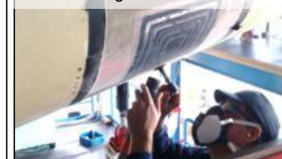
Skin perforation and two stringers disbonded
